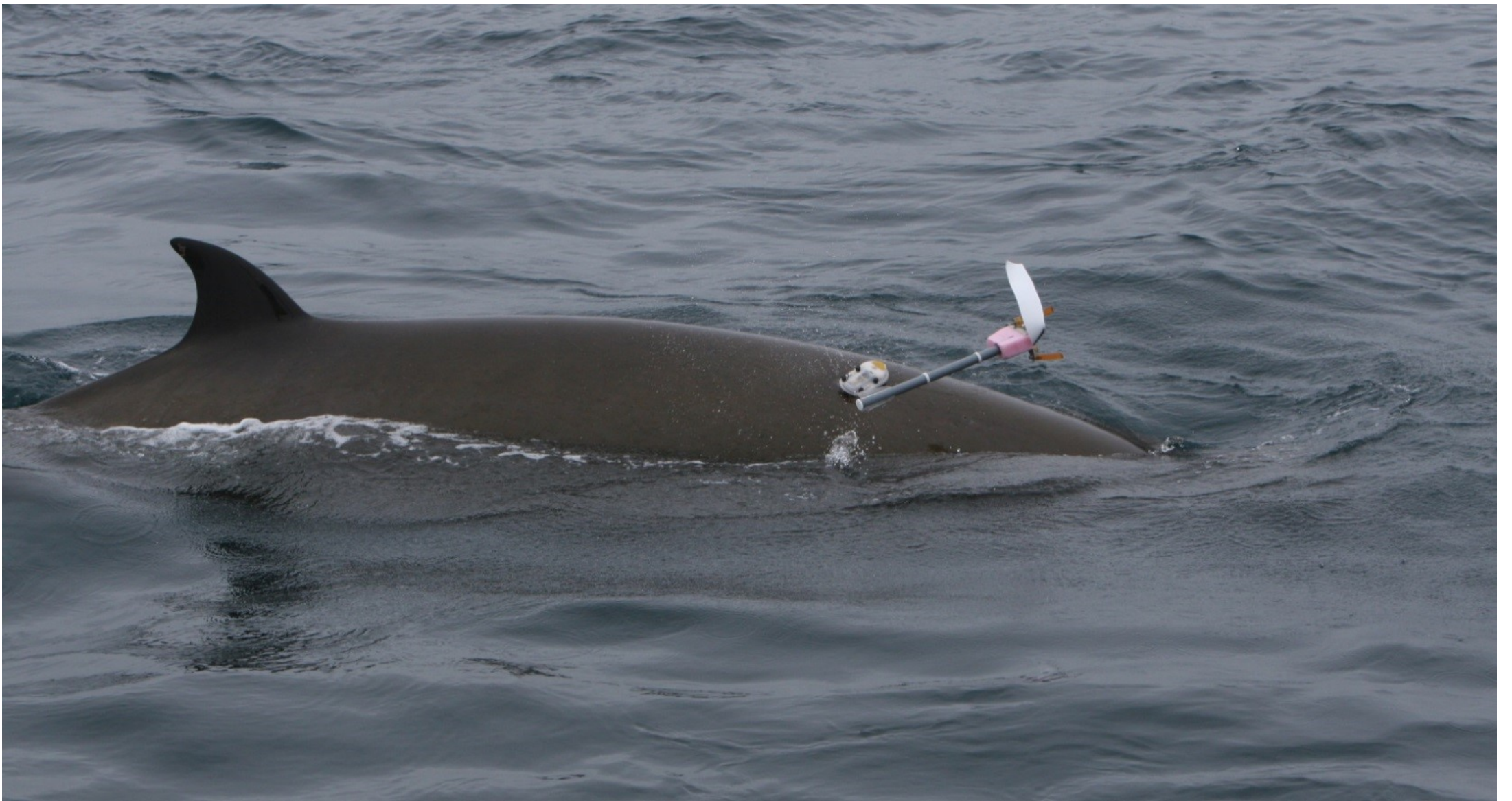
Dtag deployed onto northern bottlenose whale at 15m distance using ARTS launching system
